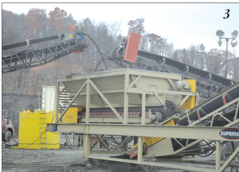
After the primary crush materials are fed to a Superior surge bin, which evens out production by leveling out the ebb and flows of material coming from the primary crusher.
