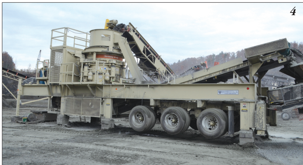
From the Superior surge bin, materials are sent to the Metso HP400 chassis mount cone crusher.
