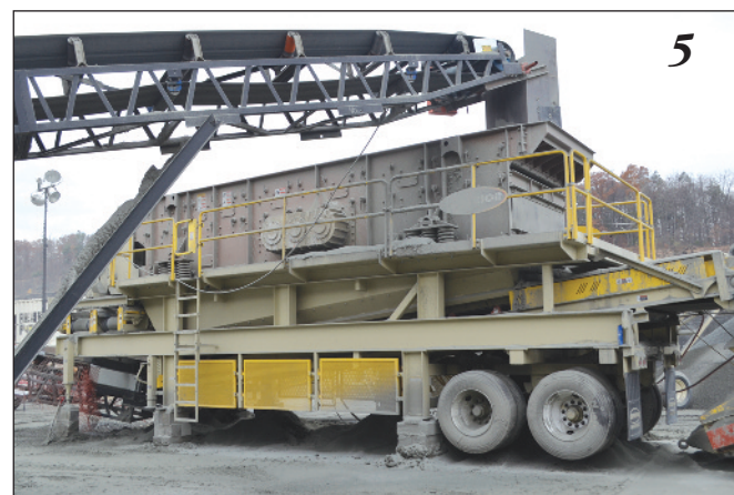
Deister 6 x 24 triple deck screener with any materials in excess of 5/8-in. (1.58 cm) being separated and sent back to the surge bin.
