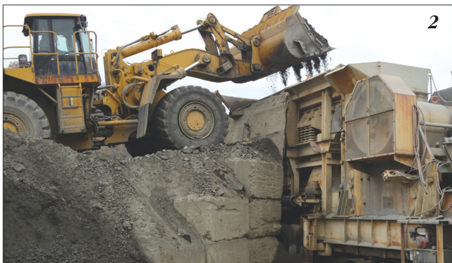
The Nordberg NW125 37 x 49 jaw receives a mixed load of material up to 36-in. (91.4 cm) minus in size.
