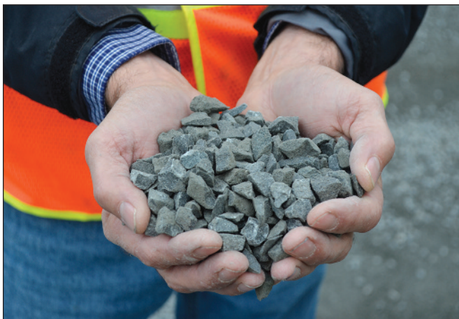
This particular rock presents its own set of challenges and makes achieving cubical particle shape very difficult.
